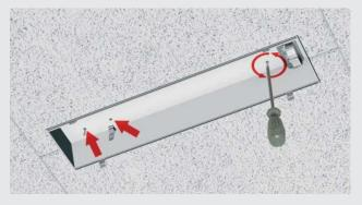
**4:** Insert the reflector and screw it tight. Press retaining clips for T5 fluorescent lamps in place.
