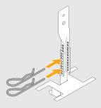
**2:** Secure the quick-hanger with nonius split-pins
