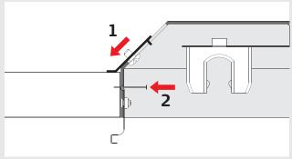
2: If it is necessary to hold the armature, punch a small nail/pin through the hole in the armature.
