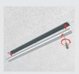
1: Install the reflector. Note: For double dishes, install the fluorescent lamp before the dish.
