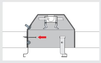
**2:** Install the transformer and then push the armature in place in the Troldtekt panel using pins.
